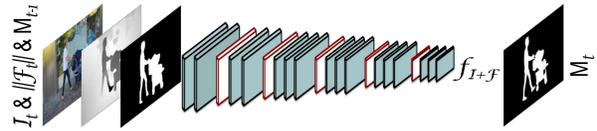
(b) One stream architecture, where 5 input channels: image  $\mathcal{I}_t$ , optical flow information  $\|\mathcal{F}_t\|$  and mask  $M_{t-1}$  are used to estimate mask  $M_t$ .
