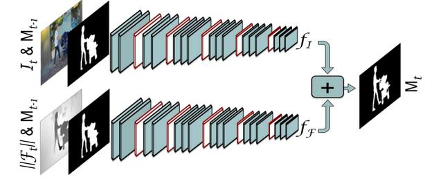
(a) Two stream architecture, where image  $\mathcal{I}_t$  and optical flow information  $\|\mathcal{F}_t\|$  are used to update mask  $M_{t-1}$  into  $M_t$ . See equation 1.
