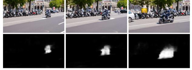
Figure 3. Video saliency results. Note that a motorcycle with motion is only focused among a lot of objects in a scene.
